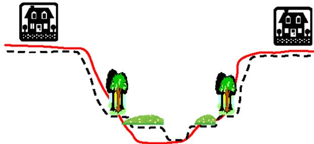
**Figure 7-15. Diagram of stepped floodplain redesign**
