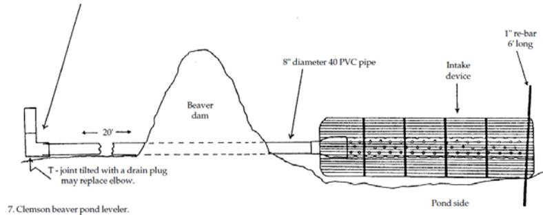
**Figure 8-4. Pond leveler to control water elevation**
