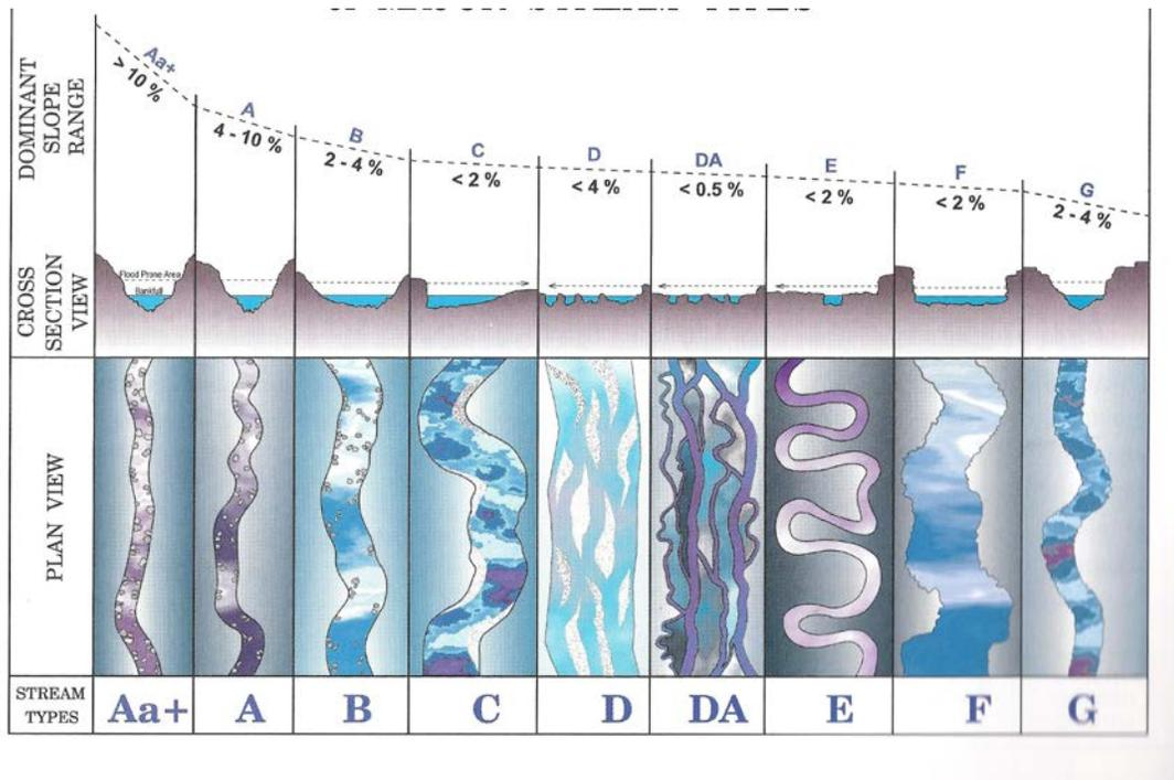
Figure 10-4. Channel types in the Rosgen classification system (Rosgen 1996)
