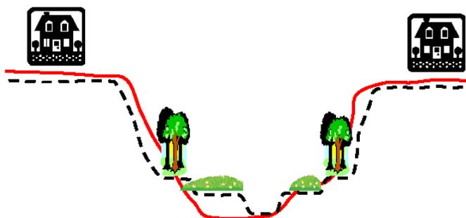
**Figure 10-11. Diagram of stepped floodplain redesign**
